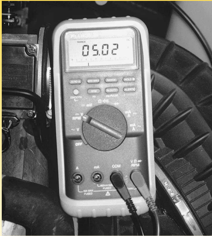
FIGURE 30-14 Checking the 5-volt reference from the computer being applied to the TP sensor with the ignition switch on (engine off).
