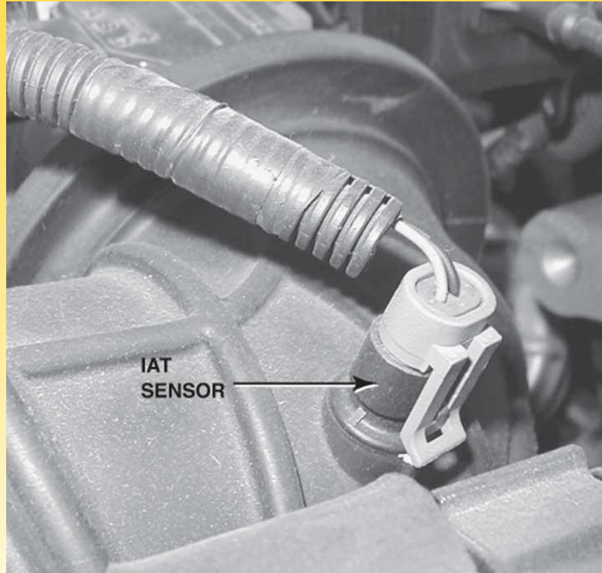
FIGURE 30-8 The IAT sensor on this General Motors 3800 V-6 engine is in the air passage duct between the air cleaner housing and the throttle plate.
