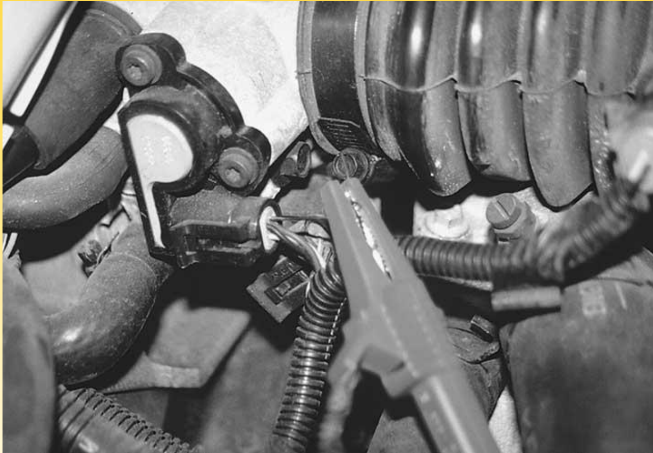
FIGURE 30-12 A meter lead connected to a T-pin that was gently pushed along the signal wire of the TP sensor until the point of the pin touched the metal terminal inside the plastic connector.
