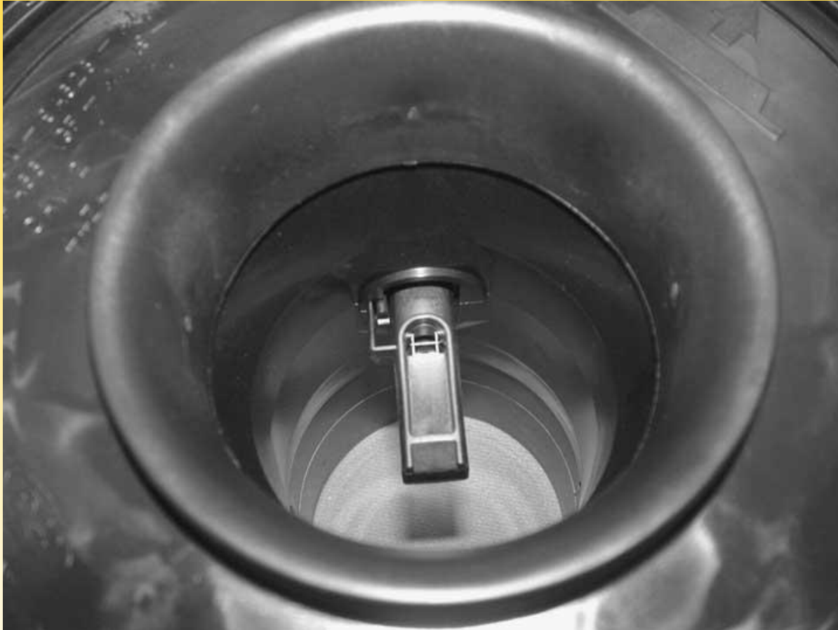
FIGURE 30-26 The sensing wire in a typical hot wire mass air flow sensor.
