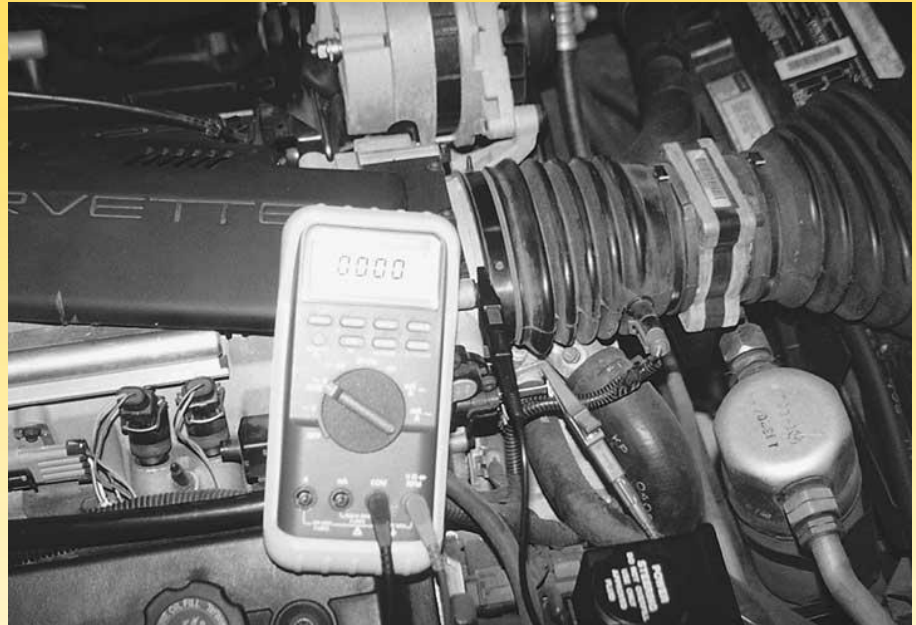
FIGURE 30-15 Checking the voltage drop between the TP sensor ground and a good engine ground with the ignition on (engine off). A reading of greater than 0.6 volt (600 mV) represents a bad computer ground.
