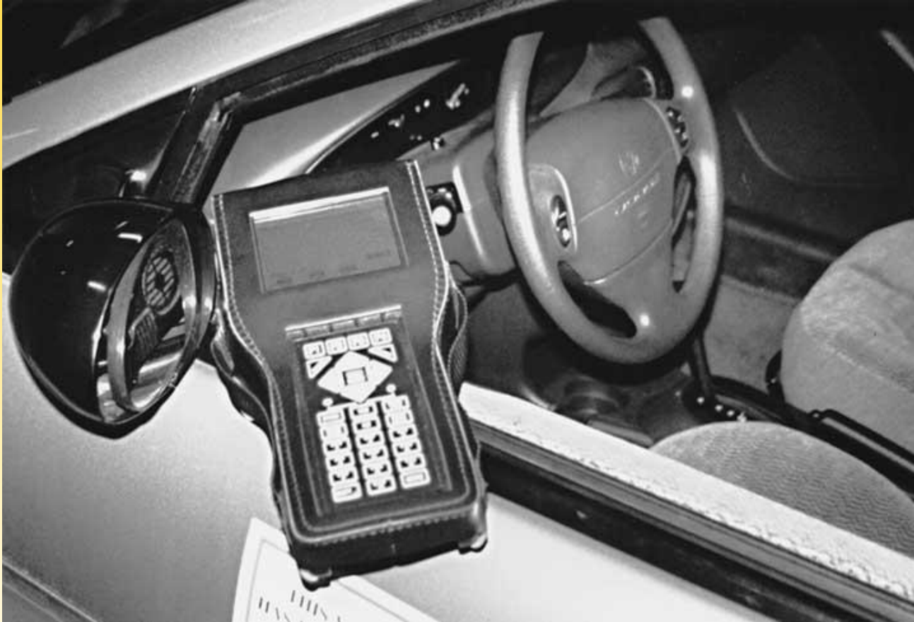
FIGURE 30-40 A Chrysler DRB III scan tool is an excellent tool to use to test an oxygen sensor(s).
