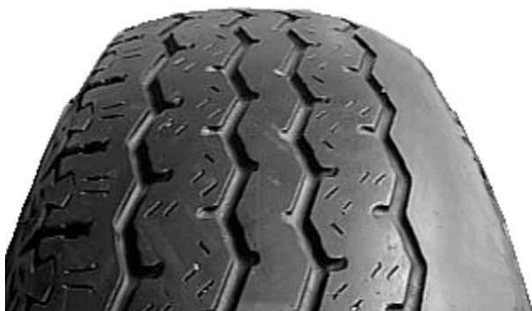
Excessive Camber Wear is isolated to the shoulder and smooth
