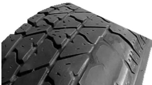
Weak Shocks or Wheel Imbalance Spotty cupping
