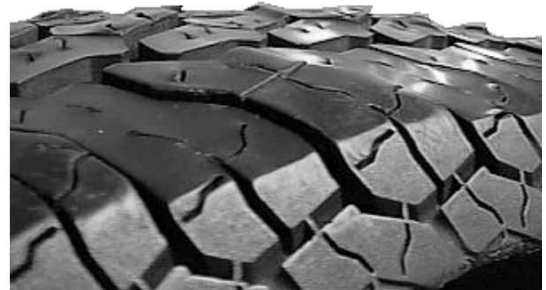
Lack of Rotation Deep front to back feathering on non-drive tires
