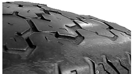
Unequal Rear Toe Diagonal wipe
