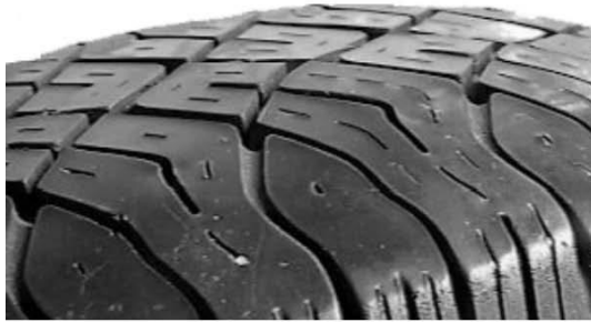
Normal Slight front to back feathering
