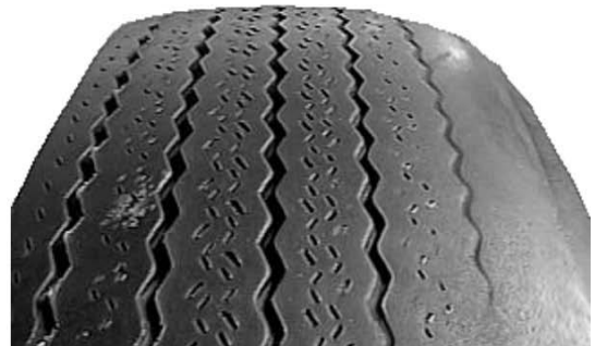
Excessive Toe Wear starts on shoulder, moves inward and feels rough
